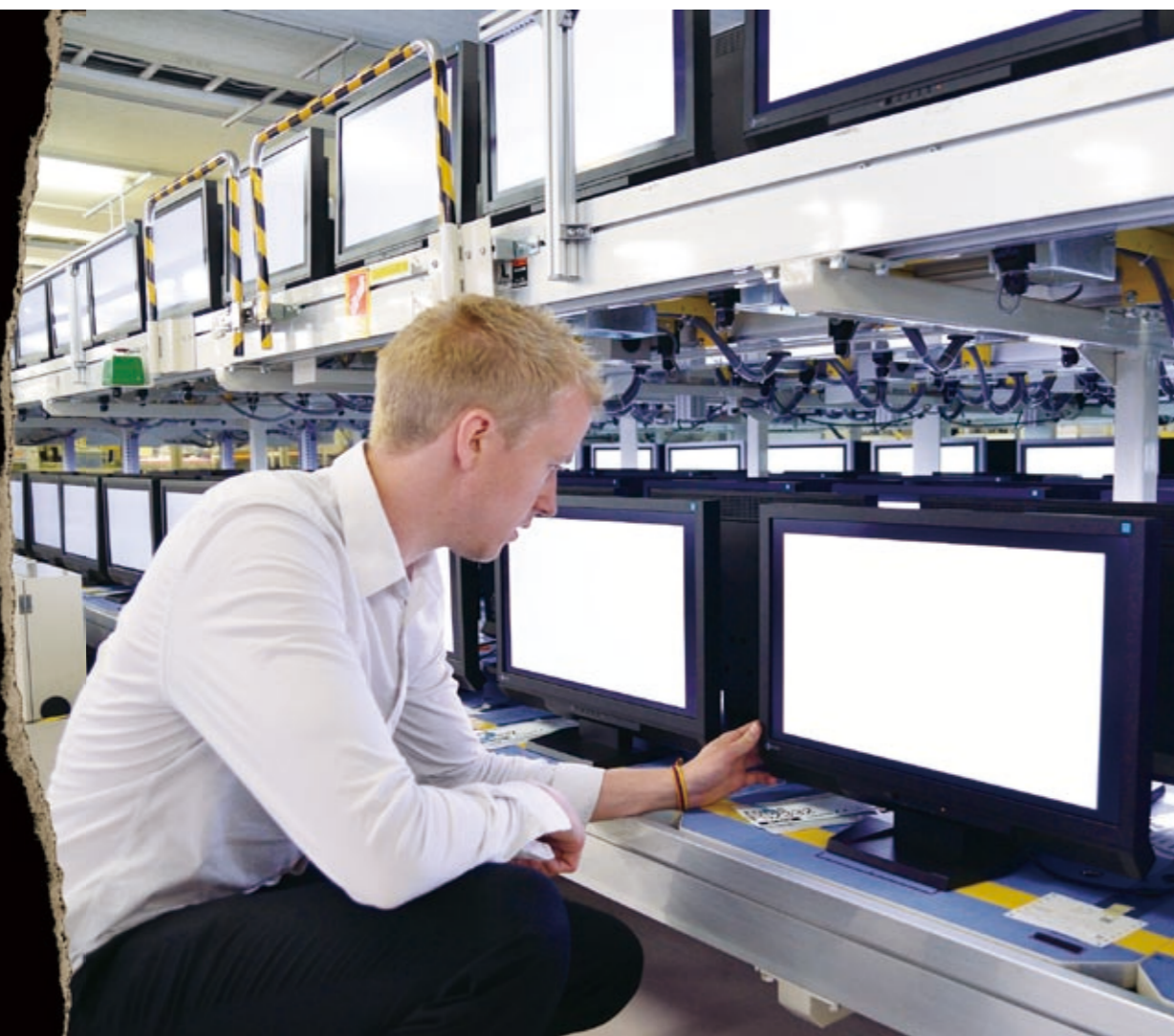
Checking out monitors undergoing the aging process, which insures that the display and electronics are stable before they are adjusted.
