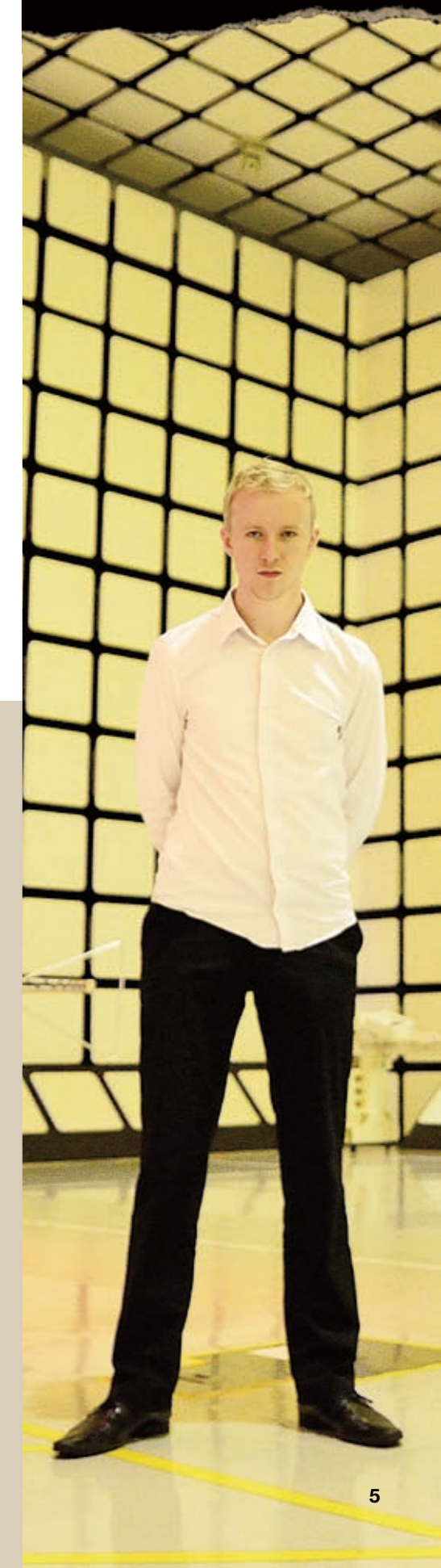
Standing in the anechoic chamber, where monitors are tested for compliance with stringent international EMC (electromagnetic) regulations.
